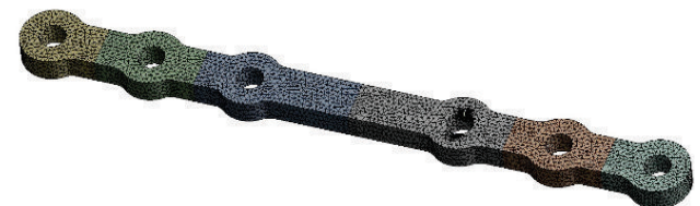
Figure 8 Plate C mesh with initial cracks
