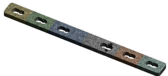
Figure 7 Plate B mesh with initial cracks
