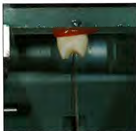
Figure 3. After demineralization, all premolar crowns were sectioned into two halves (buccal and oral) with a low-speed diamond saw under water cooling
