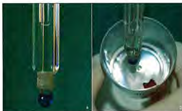
Figure 4. The pH of the demineralizing solutions was evaluated daily to maintain the initially defined values
